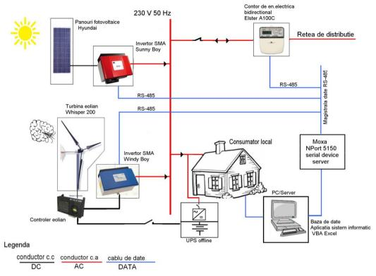
Fig. 3 - Hardware implementation of a solar-wind hybrid power system
