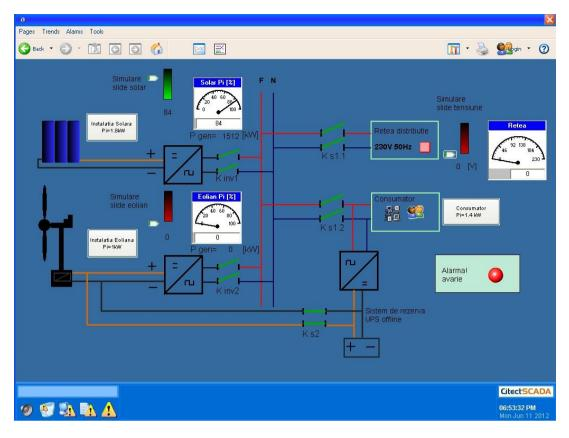
Fig. 5 - Alarm status of the hybrid solar-wind system implementation in SCADA
